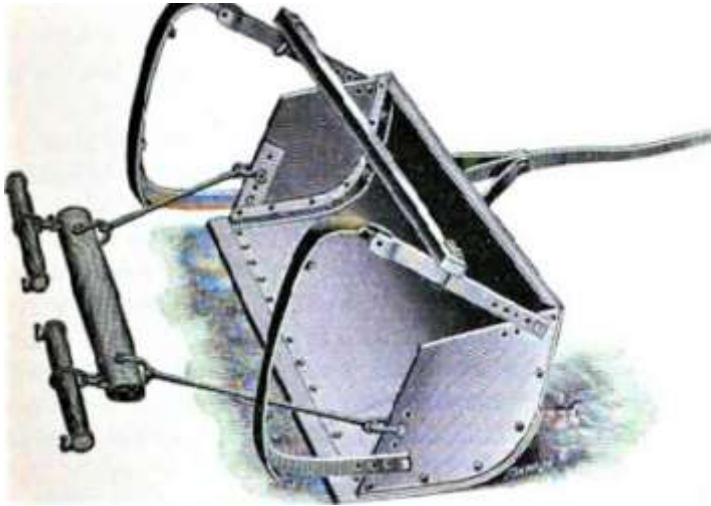
Figure 91 Drawing of early 20th-century Fresno Scraper.
