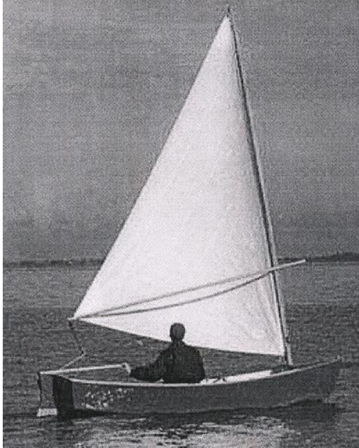
Figure 32 A skiff, with its characteristic square bow, rigged for sailing.
