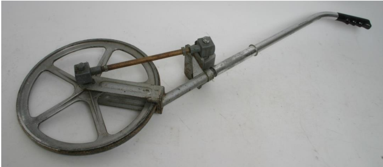
Figure 5 This antique folding metal surveyor's wheel would have been the kind of device used for measuring the yardages of the golf holes at Napanee Golf Club a century ago. Each revolution of the wheel would take one yard, and a measuring device would record each revolution of the wheel.
